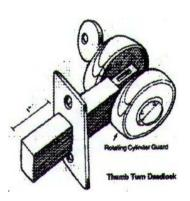
The best defense for a good solid core wood door is a deadbolt lock with one-inch throw bolt. If there are no windows in or near the door the bolt may be operated from inside by a thumb turn.
